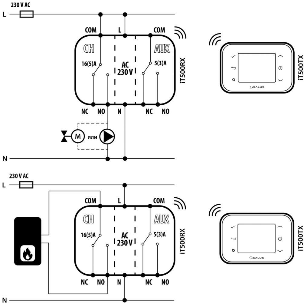
Схема подключения для двух отопительных зон
